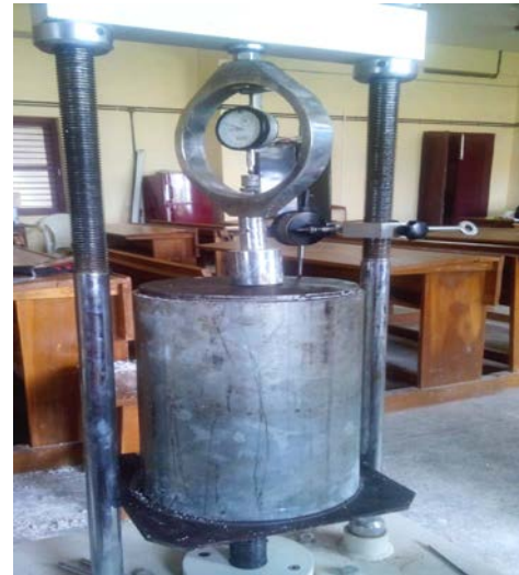
Figure 3: Test set up for Load – Settlement.
