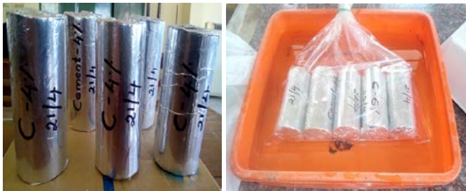
Figure 2: Wrapping and curing of specimen for unconfined compression test.
